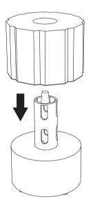
**Step5.** Put on the top cover, connect the oxygen pipe to the intake pipe in the middle and the filter is ready to use.
